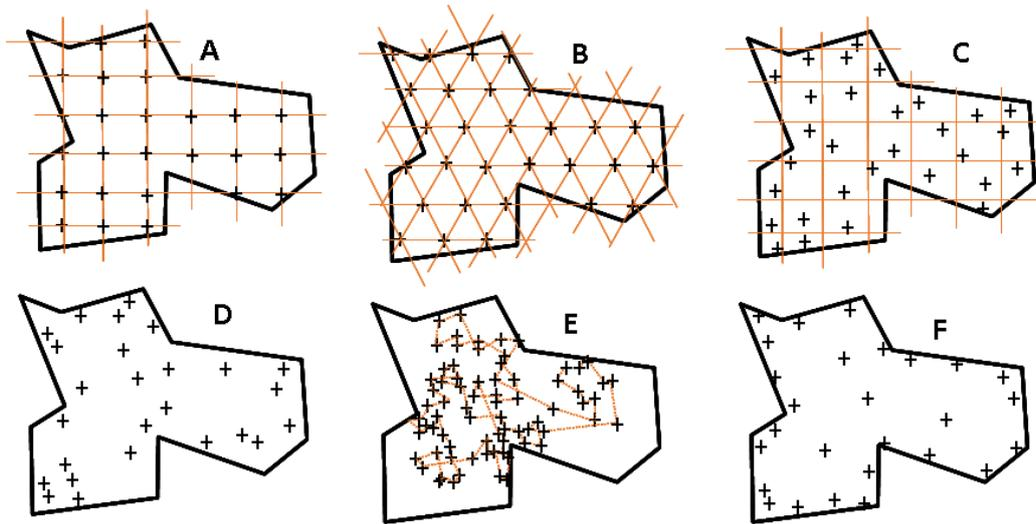
**Figure 4: Sampling patterns (see text). A – regular quadratic grid; B – regular hexagonal grid; C – stratified random; D – random; E – constrained random walk; F – preferential.**
