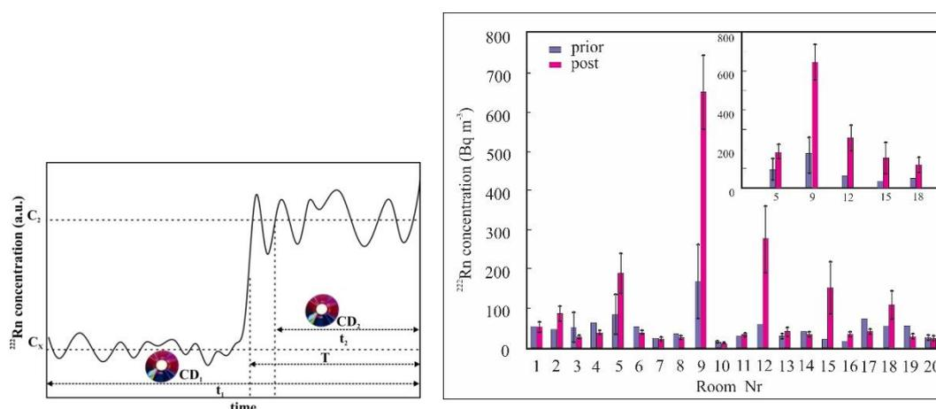
Figure 3. Concept of the CD/DVD method (left) and results of radon measurements in rooms before and after the energy efficiency reconstruction (right).
