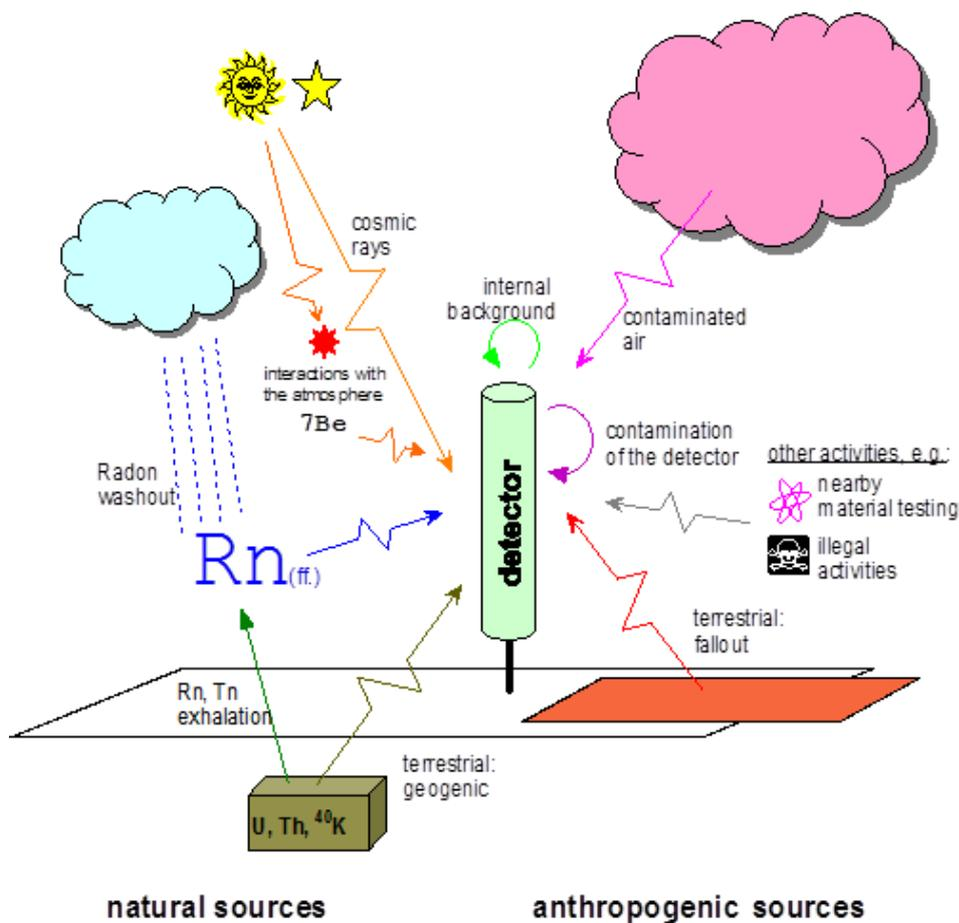
Figure 8: Contributions to the dose rate recorded by a detector. (Graph taken from the AIRDOS report).
