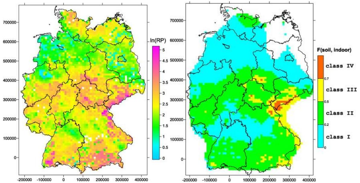
'Neznal-type' radon potential map (right) and joint distribution of radon in soil and ground floor indoor radon (left) (Gruber et al. 2013)
