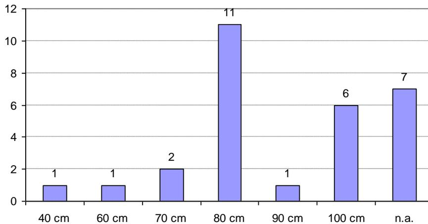
Figure 4. Standard sampling depths for soil radon measurement
