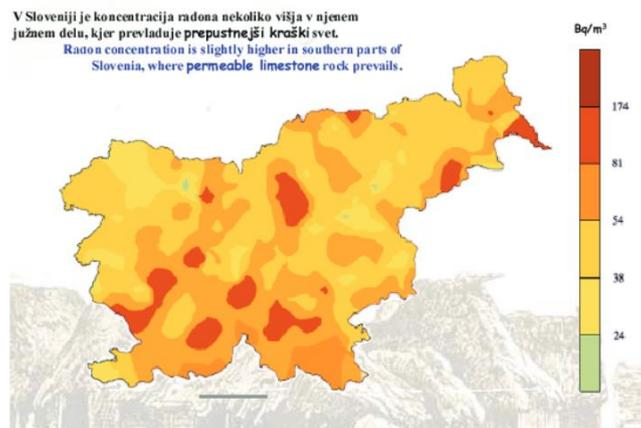
Map of indoor annual average radon concentration by interpolating the values on a grid with a resolution of 2 km × 2 km by universal kriging with linear drift (Dubois 2005).
