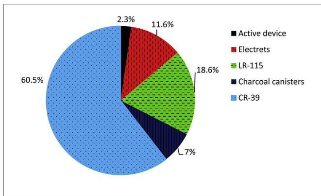
Fig. 3. Overview of used techniques for radon surveys.
