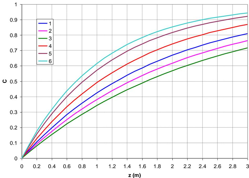
Figure 3: Radon profiles in soil for different migration parameters (Table 4)
