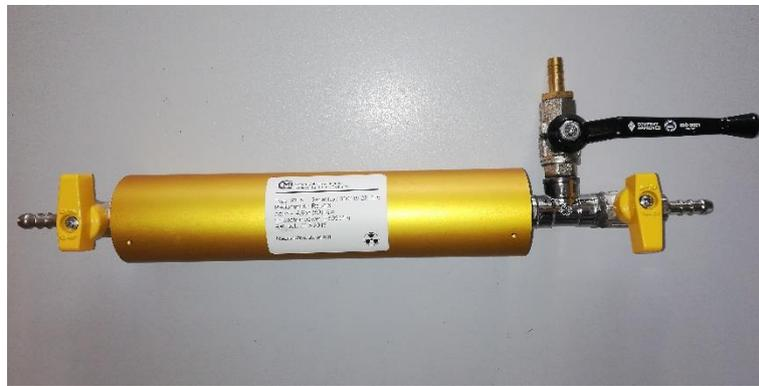
Figure D.4 The flow-through low-level radon source developed by the CMI.
