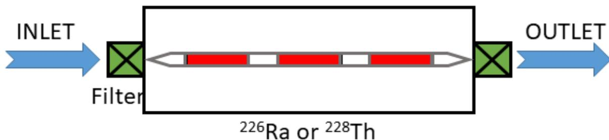
Figure 10 – New design of the source holder.
