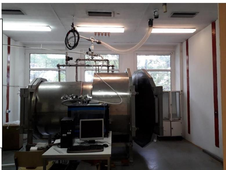
**Figure C.5.** The radon chamber from IFIN-HH: 3D concept design (left), photo (right)
