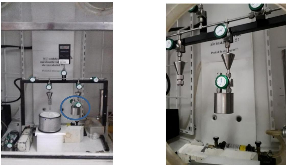
**Figure C.4.** A stainless steel recipient used for radon extraction, storage and transfer
