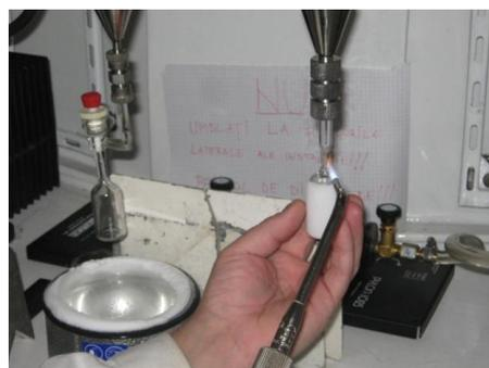
Figure C.2. The sealing of an ampoule with liquid scintillator after the radon transfer in the solution.
