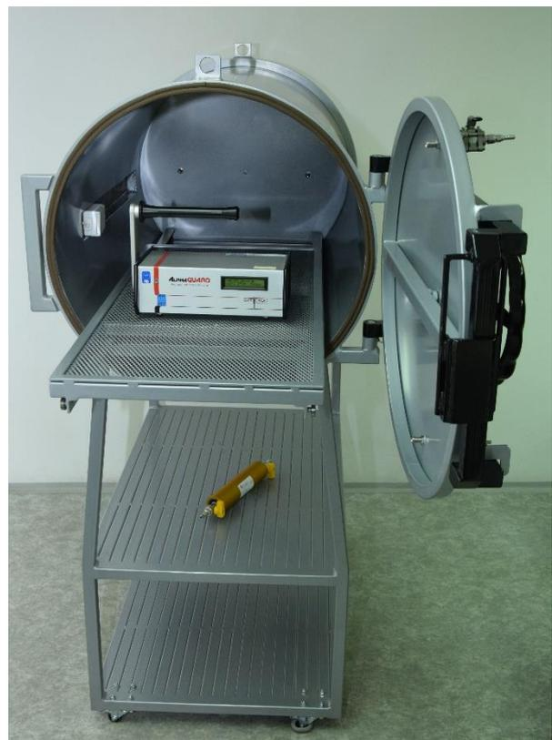
Figure D.1 The SUJCHBO Low-Level Radon Chamber
