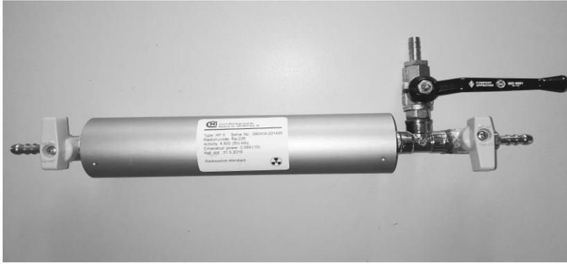
Figure 1 - The flow-through low-level radon source developed by CMI
