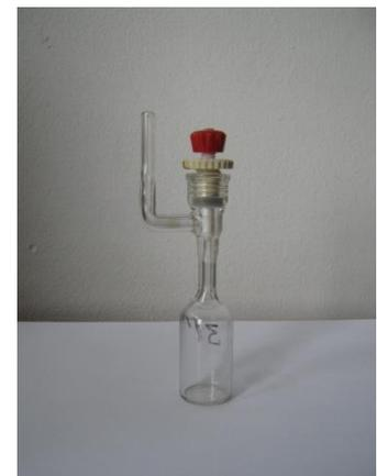
Figure C.1. The radon standard system at IFIN-HH (left); glass vial with radon (right)
