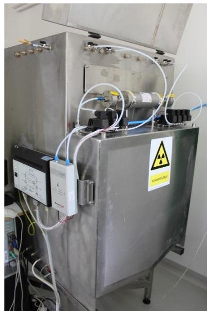
Back part with radon source and buffer
