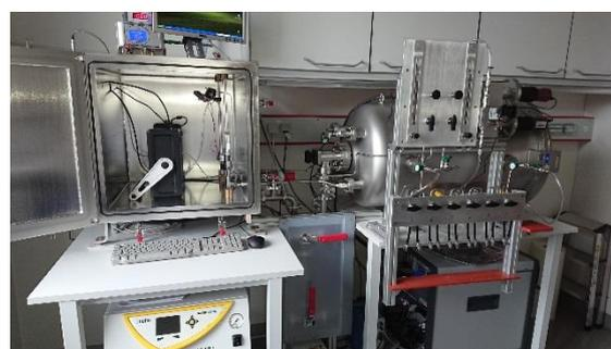
**Figure A.9.** View of the calibration facility, the calibration object from type AlphaGUARD is placed in the secondary chamber
