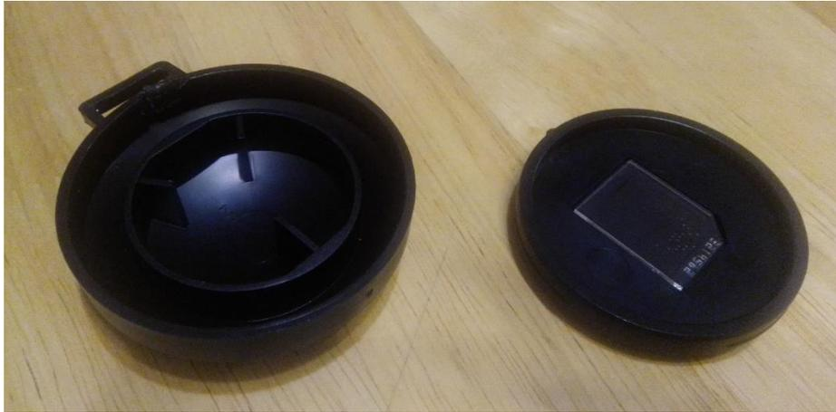
Figure 7 – An open Radtrak<sup>2</sup> detector.
