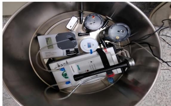
Figure A8. Snapshot of the SUBG experimental system with the reference instrument (AG).
