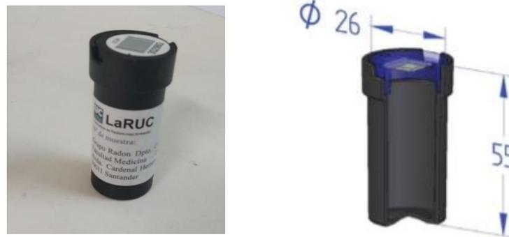
Figure 2 – RSKS passive radon detector. The indicated dimensions are in mm. (source: <http://www.radosys.com/rsks.htm>)
