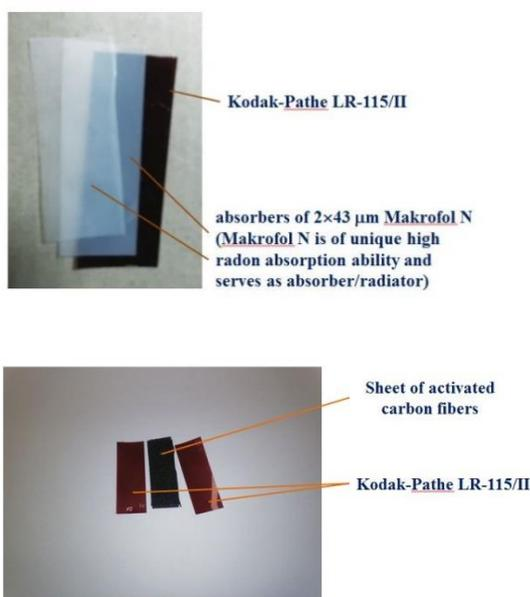
Figure 13 – Radon detectors with Makrofol N absorbers (up) and sheet of activated carbon adsorber (down) used as radiators for Kodak-Pathe LR-115/II alpha track detectors coupled with the radiators.
