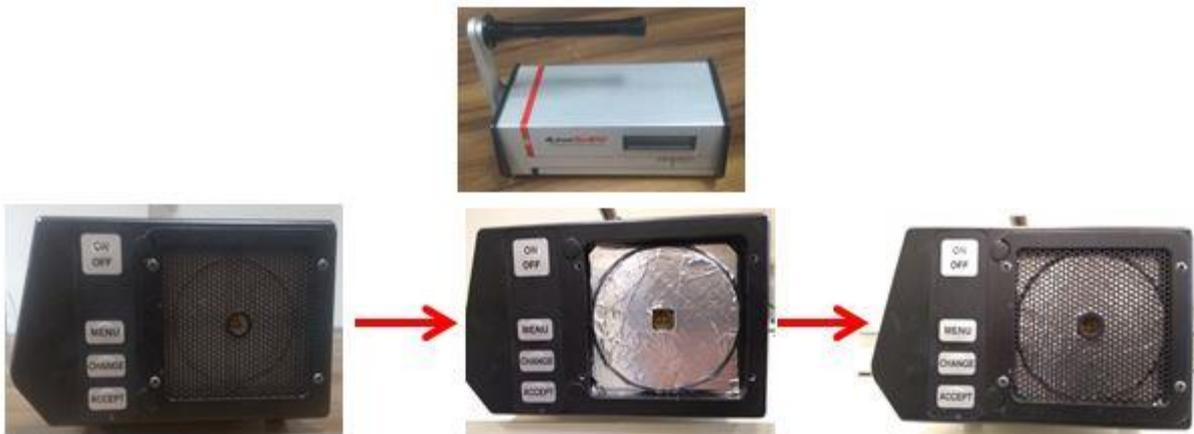
Figure 16 – Reducing thoron interference of radon monitor in a passive sampling mode by adding an additional diffusion barrier.
