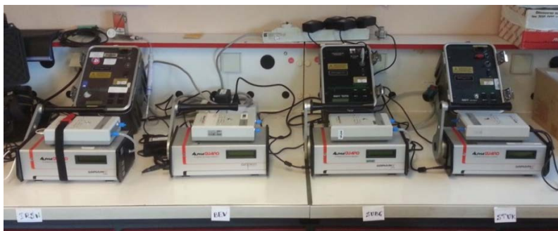
Fig.1: Preparation of the secondary reference instruments for the calibration Arrangement of the detectors in the radon chamber just before the start of the calibration.
