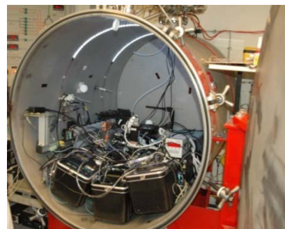
Fig.1: Preparation of the secondary reference instruments for the calibration Arrangement of the detectors in the radon chamber just before the start of the calibration.
