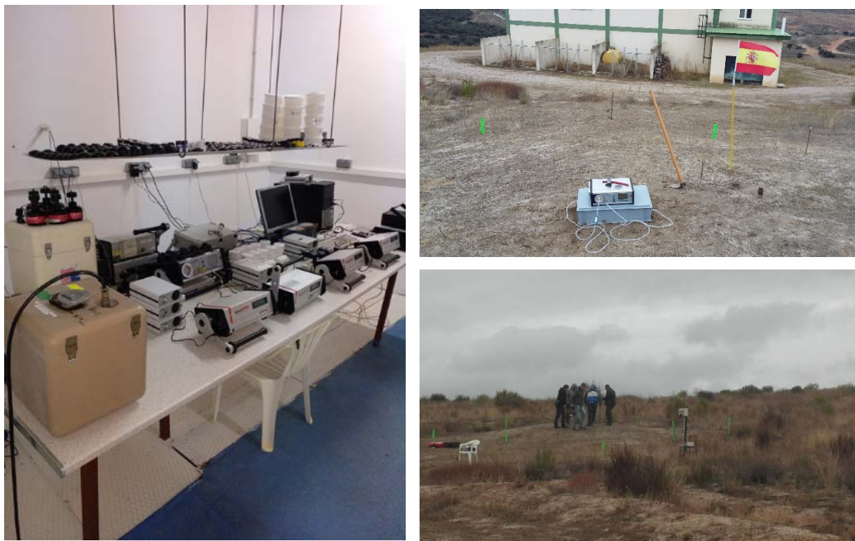
Figure 6: Left: Exposure of the passive and active monitors in the laboratory; Right top: radon exhalation measurements; Right bottom: radon in soil gas measurements; Area surrounding the laboratory of Natural Radioactivity (LNR), Ciudad Rodrigo, Spain
