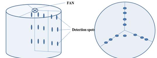
Fig. 6. The picture shows the spots in the chamber volume from where activity can be detected by the placed in a grid Kodak Pathe LR-115/II detectors.
