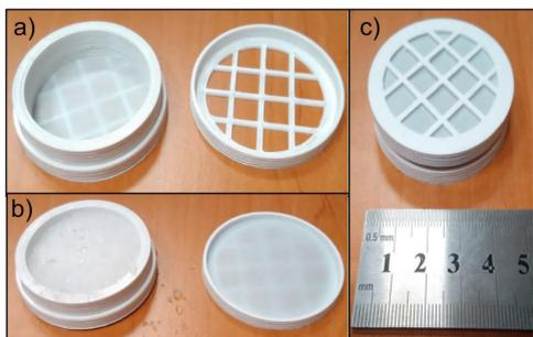
Fig. 1. Photos of a thoron sampler. a) Empty sampler ready to be filled with silica aerogel; b) the sampler filled with aerogel; c) closed sampler ready to be placed in a thoron chamber.
