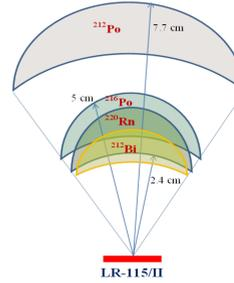
Fig. 5. Air-volumes from which alpha particles can be detected by LR-115/II detectors.
