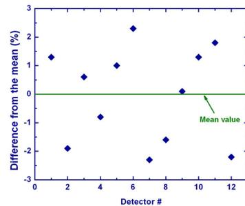
Fig. 4. Study of the repeatability of  $^{220}\text{Rn}$  homogeneity evaluation with thoron samplers. All results are within  $\pm 2.3\%$ .
