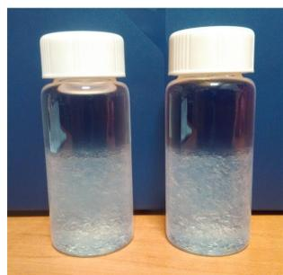
Fig. 2. High performance LS glass vials (20 mL) filled with silica aerogel and Ultima Gold LLT LS cocktail.
