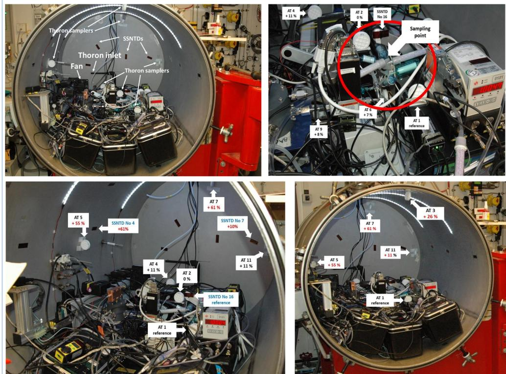
Fig. 7. Thoron homogeneity study during the BACCARA calibration exercise.
