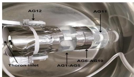
Fig. 3. Photograph of the exposure set-up used to test the repeatability of the method. The fan and the tube with the samplers are placed in a 50 L vessel.
