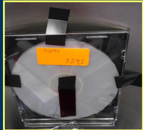
DVD surface with Makrofol N absorber
