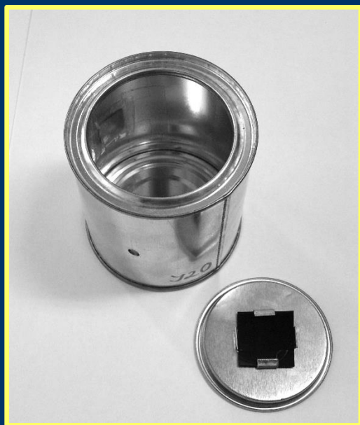
SUBG metal chambers with Kodak LR-115/II
