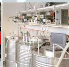
Left: inside view of the IRSN (France) radon/thoron chamber, right: stainless steel containers for the calibration of radon instruments at BfS (Germany).
