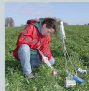
Taking a sample for soil gas radon measurements.
