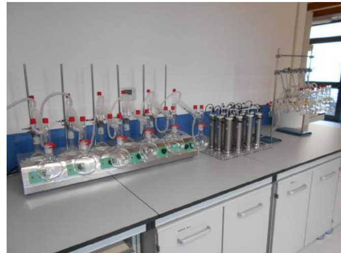
Tritium Enrichment used in combination of beta spectrometry (tritium contents in water)
