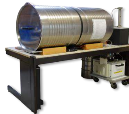
Complete calibration facility with 300 l calibration container, 30 l active coal filter and radon source
